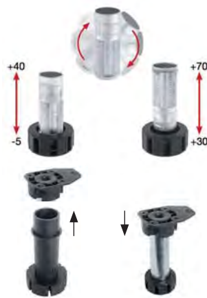
Remove base adjusters top fitting and place in adjuster
